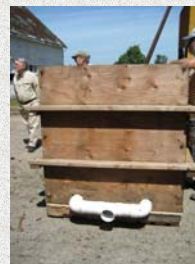
Fig. 2. 2.5-yard aerobic reactor showing aeration pipes and pump connector
